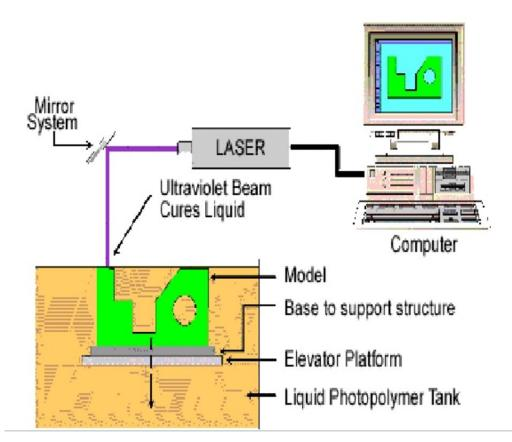
Stereo lithography is an additive manufacturing process using a vat of liquid UVcurable photopolymer "resin" and a UV laser to build parts a layer at a time.
