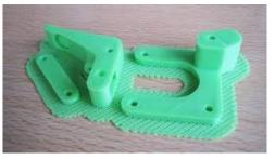
Supports: Supports are vertical scaffolds intended to be removed and discarded: They are added when there is a hole or extrusion that will collapse under gravity.
