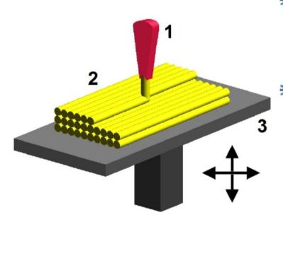
**Fused deposition modeling** (FDM) is an additive manufacturing technology commonly used for modeling, prototyping, and production applications.
